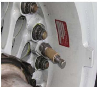
SmartStem Tire Pressure Sensor installed
