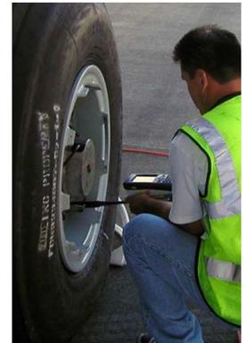
1. HandHeld Reader (HHR) communicates wirelessly to **SmartStem** Tire Pressure Sensor (TPS)
